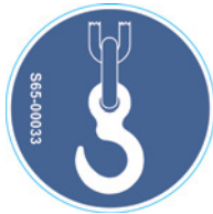
Indicates lifting points on the drill
