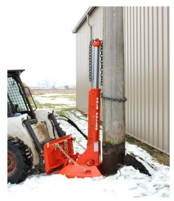
5) Extend the Utility Pole Puller cylinder to lift the pole out of the ground. The chain/wire rope will choke around the pole as the cylinder extends and pull the pole out of the ground.
