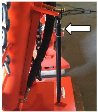
Remove Lynch Pin (arrow above) from Cylinder Strut before engaging the cylinder to pull the pole out of the ground.
