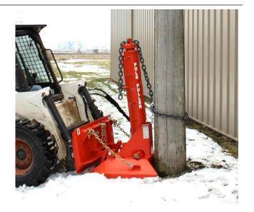
2) Position the Utility Pole Puller as close to the pole to be removed as possible. This will enable more lifting power and will remove the pole quicker.
