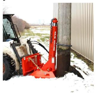
Lower the cylinder back down. The chain/wire rope should loosen and drop back down.
