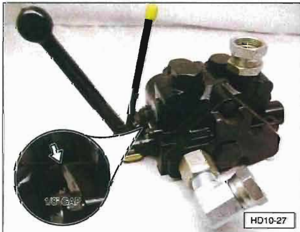
Gap Between Setscrew and Valve Body.
