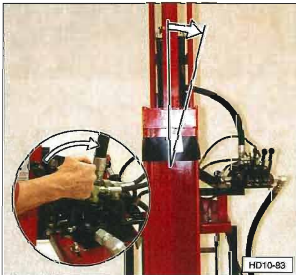
Tilt Top of Drive Ram Toward Operator.
