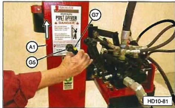
(A1) Drive Ram. (G5) Hydraulic Control Valve Lever. (G7) Safety Lever.
