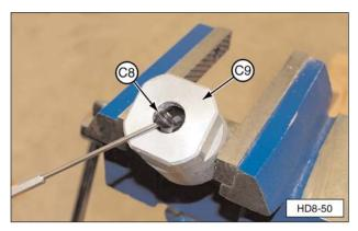
(C8) Cylinder Cap. (C9) Cylinder Cap Seal.
