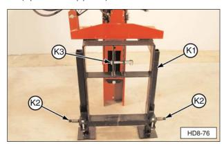
(K1) Three-Point Hitch Weldment. (K2) Leg Bracket Weldments. (K8) Stabilizer Leg Lock Bolt.
