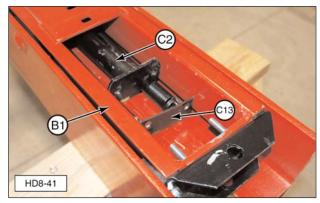
(B1) Main Carriage Channel. (C2) Drive Cylinder. (C13) Spring Bracket.
