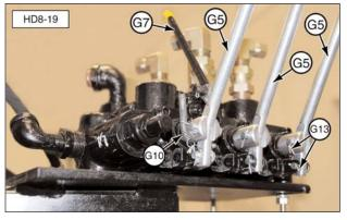
(G5) Control Valve Lever(s). (G7) Control Valve Safety Lever. (G10) Safety Lever Return Spring. (G13) Cotter Pin(s).
