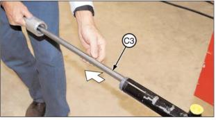
(C3) Cylinder Piston Rod. (C7) Cylinder Cap.
