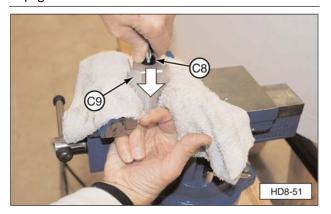
(C8) Cylinder Cap. (C9) Cylinder Cap Seal.
