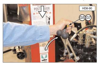
(G5) Control Valve Lever. (G7) Control Valve Safety Lever.
