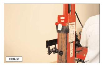
**19.** Squeeze control valve safety lever (G7) and push control valve lever (G5) to release the drive ram and create impact.
