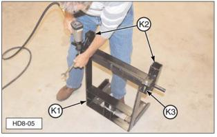
(K1) Three-Point Hitch Weldment. (K2) Leg Brackets. (K3) Leg Bracket Bolt.
