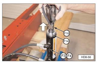
(F3/F4) Cylinder (forward or side tilt). (F14) Internal Cylinder Cap Snap Ring. (F16) Cylinder Rod Assembly.
