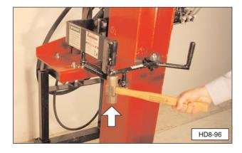
**9.** Install Lynch pin to secure swing arm to the safety arm frame.
