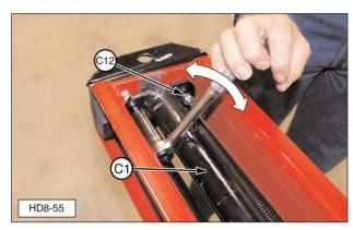
(C1) Hydraulic Drive Cylinder Assembly. (C12) Self Locking Nuts.
