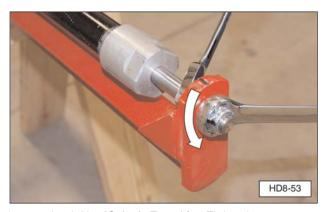
Loosen Lock Nut (C4) 1/2 Turn After Tightening.
