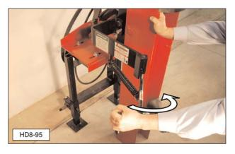
8. Tap swing arm handle shaft up through safety arm frame tube. Install Lynch pin (I13) to secure the swing arm to the safety arm frame.
