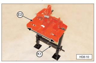
(E2) Manual Base Plate. (K1) Three-Point Hitch Weldment.
