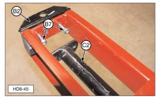
(B2) Road Lock Bracket. (B7) Road Lock Bracket Nuts. (C2) Drive Cylinder.
