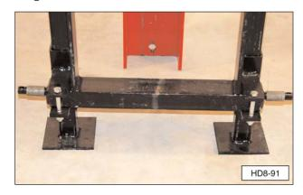
**3.** Raise or lower the stabilizer legs to allow drive ram I-beam full contact with the ground. Make sure the Post Driver is stable.
