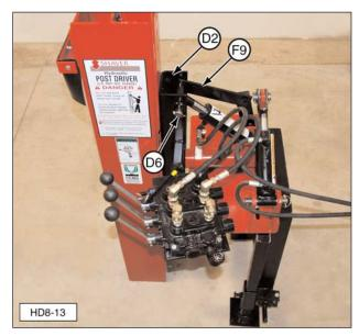
(D2) Short Channel Bracket (hydraulic).(D6) Channel Mounting Pin. (F9) Safety Lever Plate.
