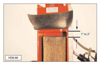
**17.** Close safety arm frame (I2) to secure the post (the adjustable roller assembly keeps tension on the post while it is being driven).
