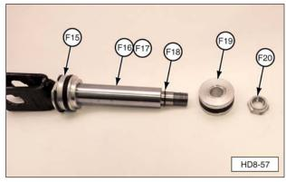
(F15) Cylinder Cap. (F16 or F17) Cylinder Rod. (F18) O-ring Seal. (F19) Cylinder Piston (with seal). (F20) Self Locking Nut.
