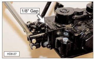
Gap Between Setscrew and Valve Body.
