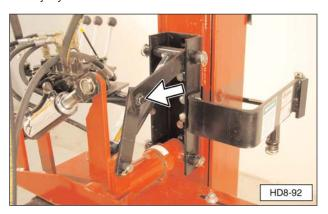
5. Make sure pressure is relieved from the Post Driver hydraulic system. Disconnect hydraulic pressure supply hose (G17) from the tractor. Disconnect hydraulic return hose (G20) from the tractor.
