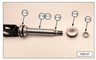
(F15) Cylinder Cap. (F16 or F17) Cylinder Rod. (F18) Cylinder Rod Seal. (F19) Piston. (F20) Cylinder Rod Nut.
