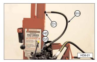
(C1) Drive Cylinder Assembly. (G1) Control Valve (Single Lever). (G15) Valve to Drive Ram Hose. (H1) Control Valve (Triple Lever) (not shown).
