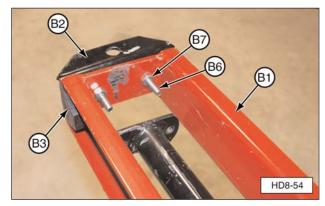
(B1) Main Carriage Channel. (B2) Road Lock Bracket. (B3) Rubber Bumper. (B6) Bolt. (B7) Nut.
