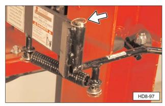
**10.** Verify the swing arm handle opens against safety arm frame (I2) stop bracket and closes against back wall of drive ram (A1) I-beam.
