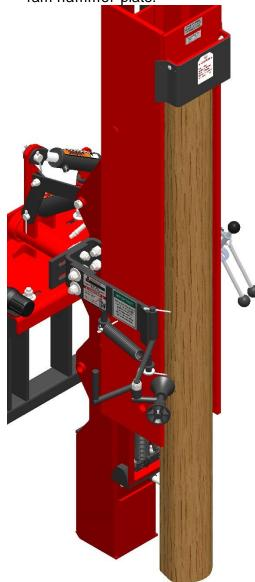
NOTE: There should be a 1" to 2" gap between the top of the fence post and the bottom of the drive ram hammer plate. Never drive a fence post without the guard in place.
