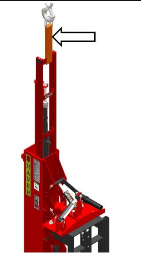
Overhead lifting device (arrow) Hydraulic Base Plate
