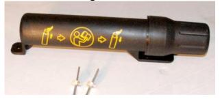
Manual Storage Tube & mounting rivets.
