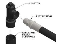
directly to the hydraulic reservoir of the tractor or skid loader.
