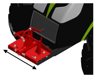
3. Install manual base plate on front mount adapter as shown. Install carriage bolts, washers, lock washers, and nuts removed in Step 1. Center the base plate on the three-point hitch and tighten the hardware securely.
