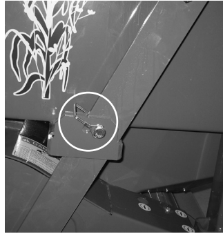
Pickup lift with travel lock pin.
