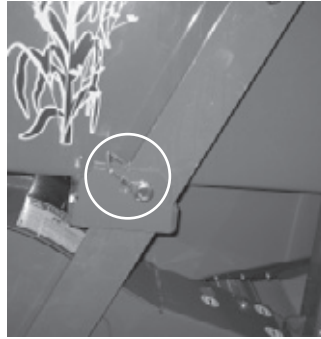
Pickup lift with travel lock pin.
