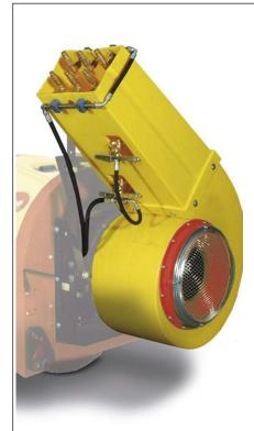
The cannon fan group has similar gear box like normal axial fan groups and the characteristics are similar too. The impeller has a centrifugal fan type capable to producing an air flow at high speed, guaranteeing a high spraying.
