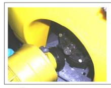
Insert the PTO shaft onto the splined shaft of the machine while holding down the safety plug
