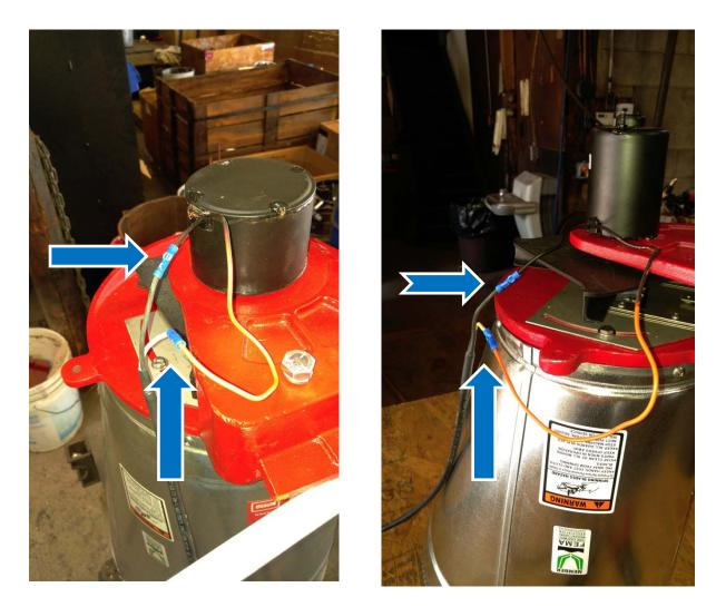
Now connect the wire labeled "motor" to the motor. Black to black. White to orange. Slide the stripped wire into the connector and crimp tight.
