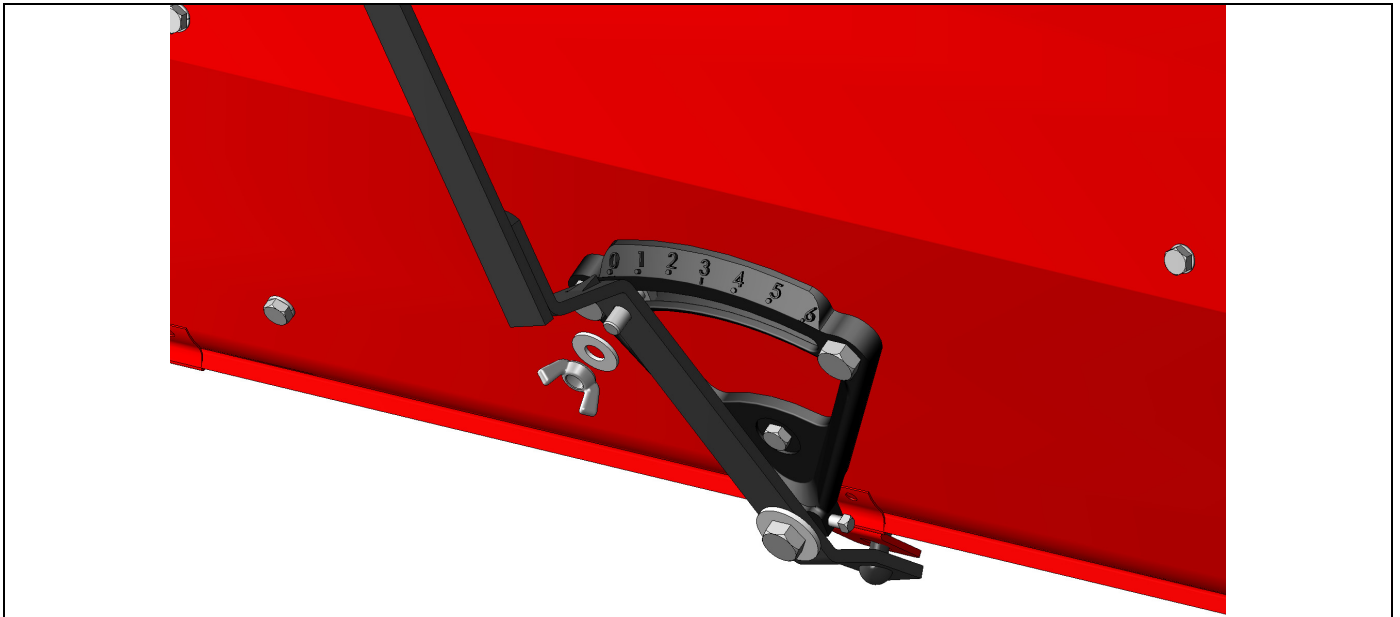
Figure 4-12: Box Slide at "0" Position
