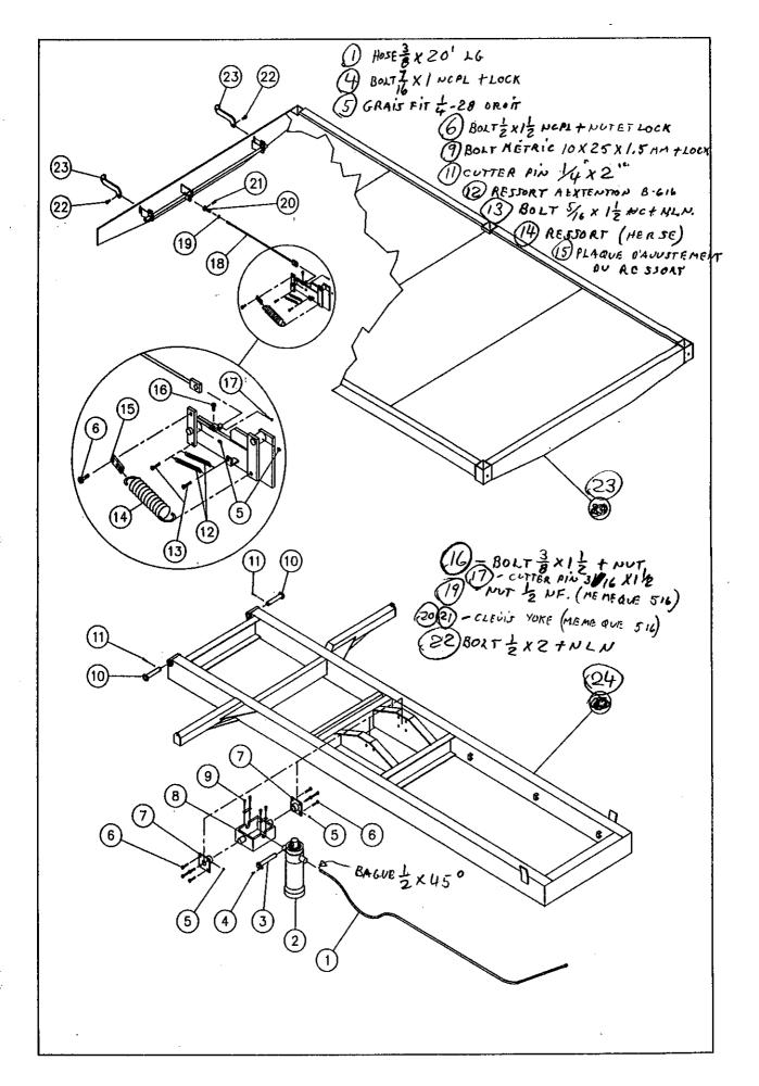
(26) BOLT & X 4 + LOCK, NUT ET FLAT. Kit MUNICAU 1648171684
