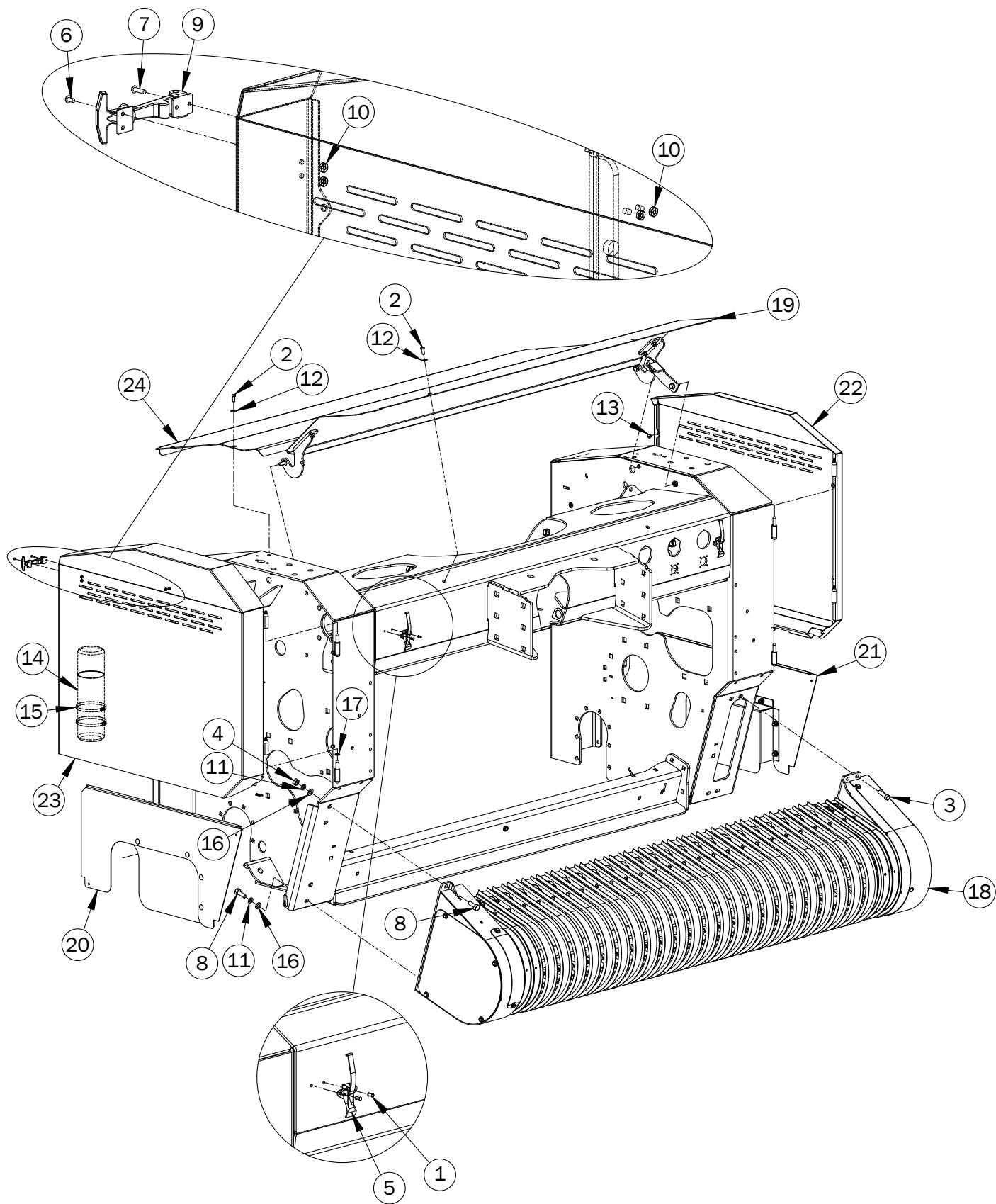
**Pickup, Guards & Shields Assembly - View A**
