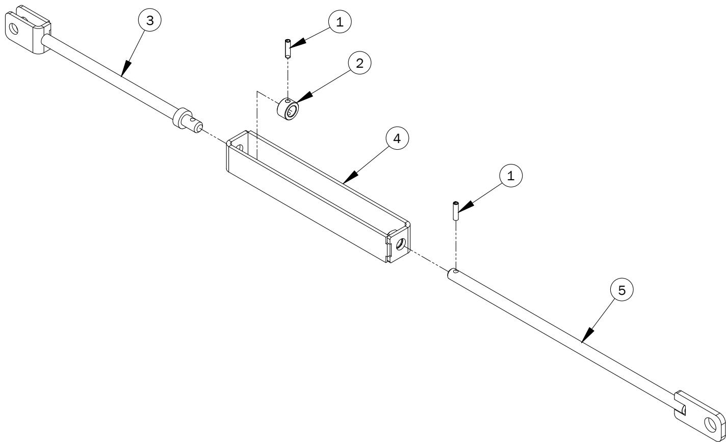
**Tedder Attachment Kit K104 Turnbuckle Assembly**
