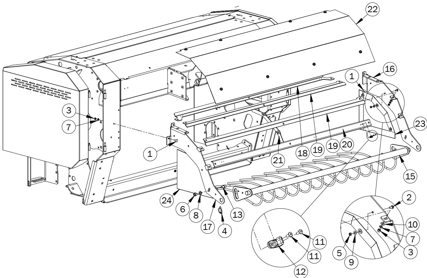
**Pickup, Guards & Shields Assembly - View B**
