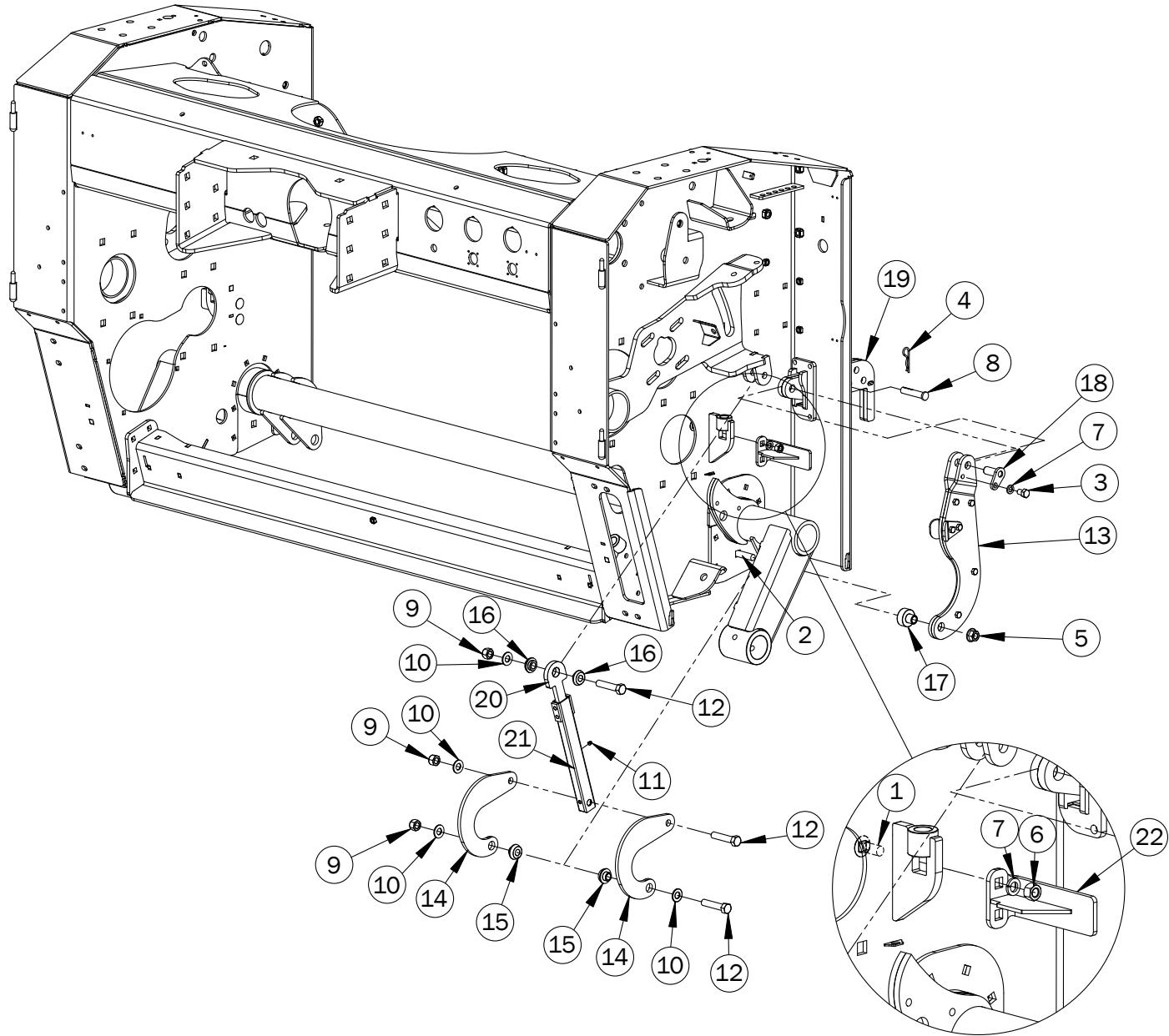
**Lift Bracket Assembly - Right & Left Sides**
