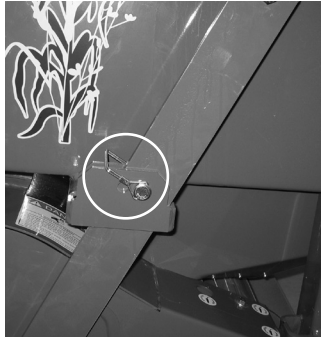
Pickup lift with travel lock pin.
