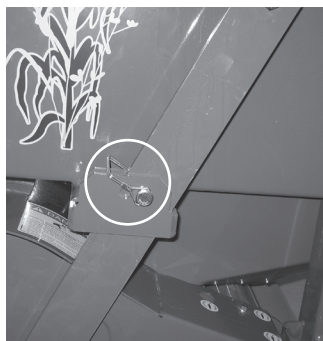
Pickup lift with travel lock pin.
