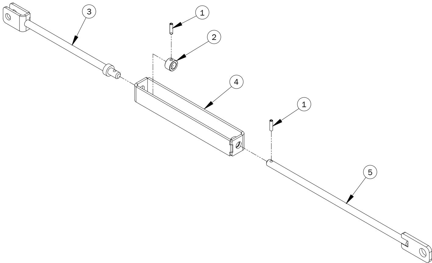
**Tedder Attachment Kit K104 Turnbuckle Assembly**
