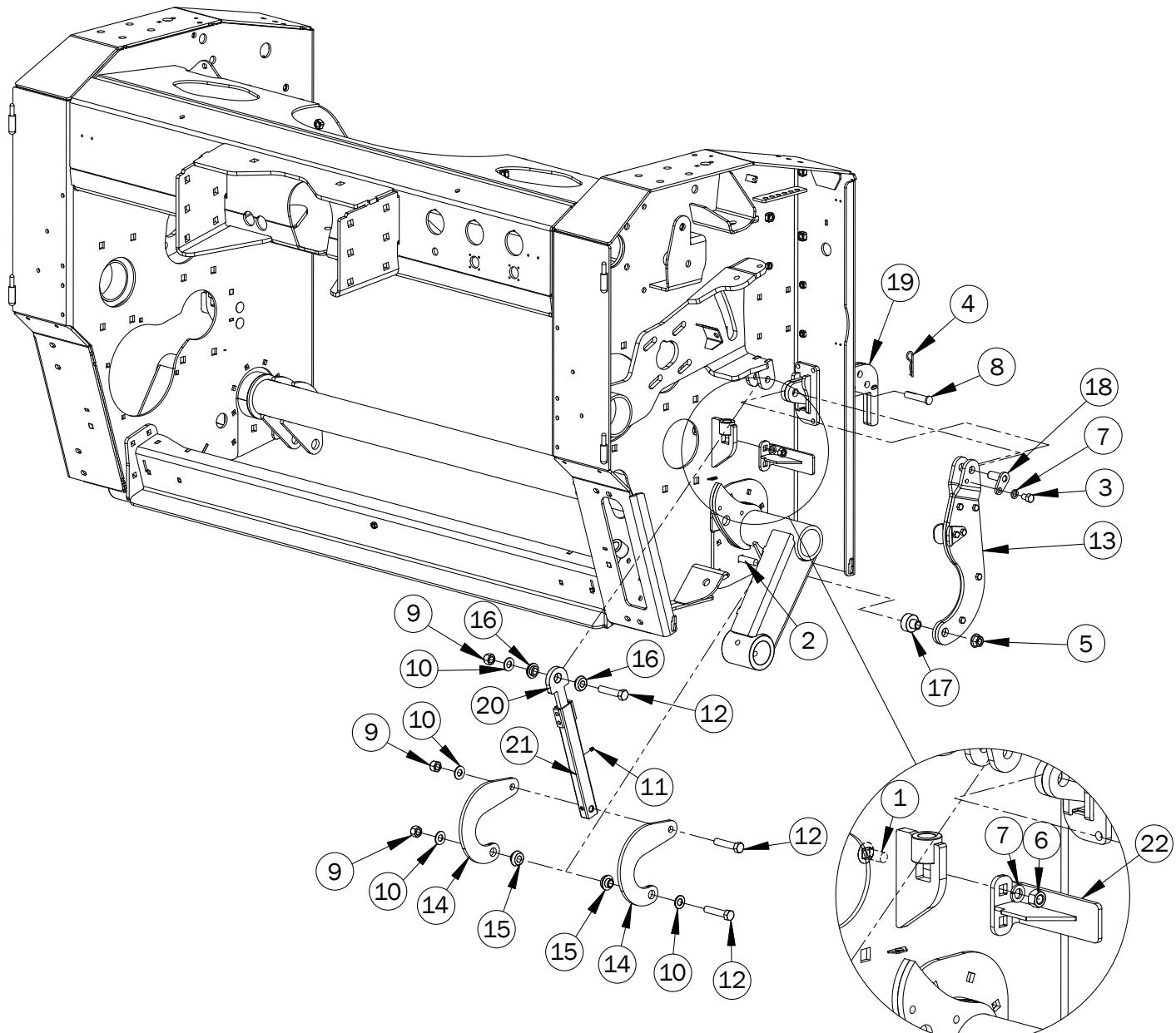
**Lift Bracket Assembly - Right & Left Sides**
