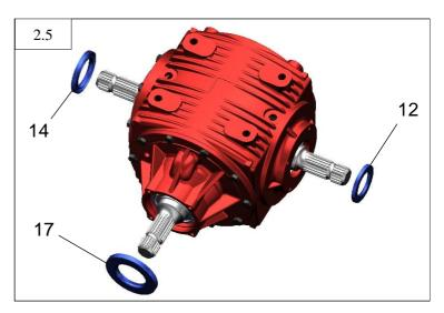
• Put a silicone film between housing and copper washer contact surfaces.
