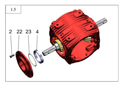
• Unscrew bolts (2) and take away cover (22), using a chisel and hammer.
