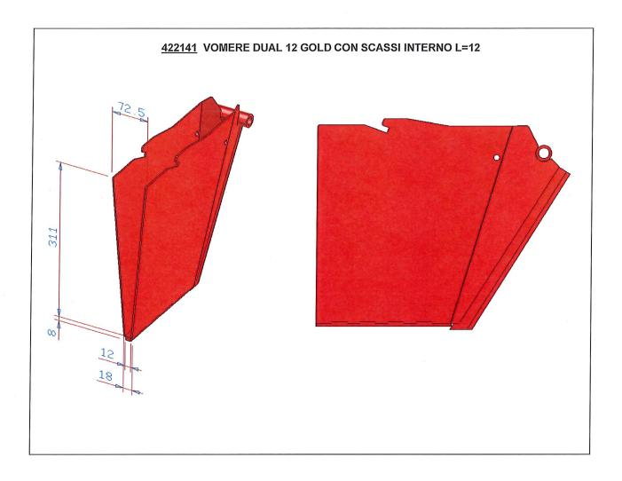
The runner above is a new runner available for the Dual 12 Gold, and is intended for very small plant plugs only. It is NOT recommended that this runner be promoted as a "standard" runner as it has the same high wear characteristics as the early Dual 12 runners. The standard runner, #421586, should still be recommended in all normal situations.
