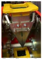
The Wolf cup is still a sturdy cup, but smaller than the WolfPRO cup and made of aluminum and harder to change out.
