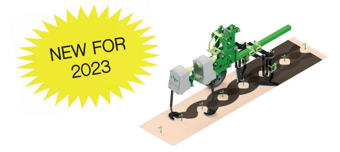
The Garford Dual eRotor System is specifically designed to have two counter rotating eRotor ground engaging shares. This will facilitate complete weed control between the crop plants, by having two opposing rotating shares, giving the added advantage of repositioning the soil from the primary rotor, prior to the InterRow shares following behind. This will also have increased aeration of the soil via the second rotor share stimulating plant growth.
