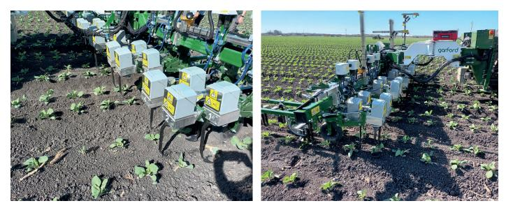
The Dual eRotor option is aimed at customers with production systems that demand very high weed control efficacy and would be double passing today, once in each direction. In these production systems the Dual eRotor option can deliver an 100% productivity increase.
