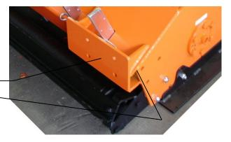
Mounting the support of the RSI on the plate on the machine
