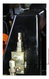
Drill two holes on the right side of the 3 point attachment and connect the max pressure valve to it.
