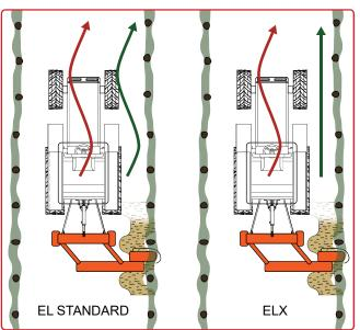
The patent device "RSA" controls the side shifting of the machine when it comes back to the trees line.
