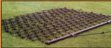
LIGHT PENETRATION Front section Tines position "B" Rear section Tines position "B"
