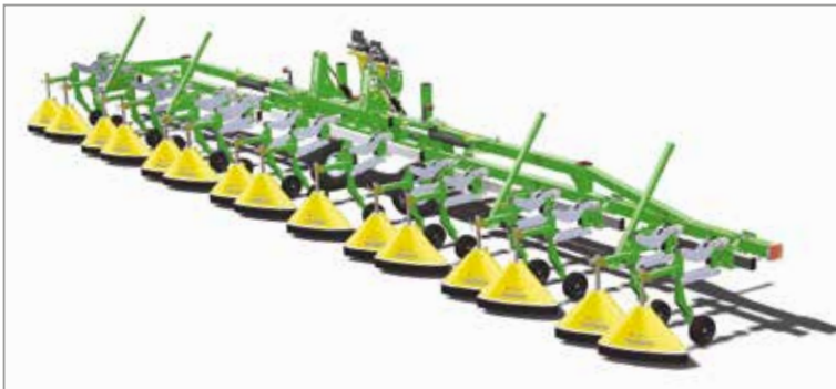
Varidome S7 with overlapping 170 HiFlo shield configuration for sugar cane.
