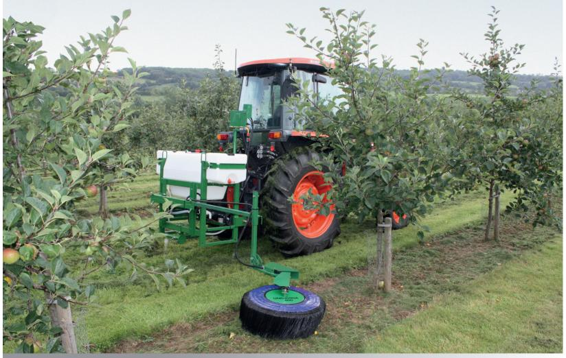
Incorporating either traditional hydraulic pressure nozzles or Micron CDA (Controlled Droplet Application) atomisers, the Undavina range of vehicle-mounted sprayers offers an efficient and targeted method of weed control round the base of vines and fruit trees.
