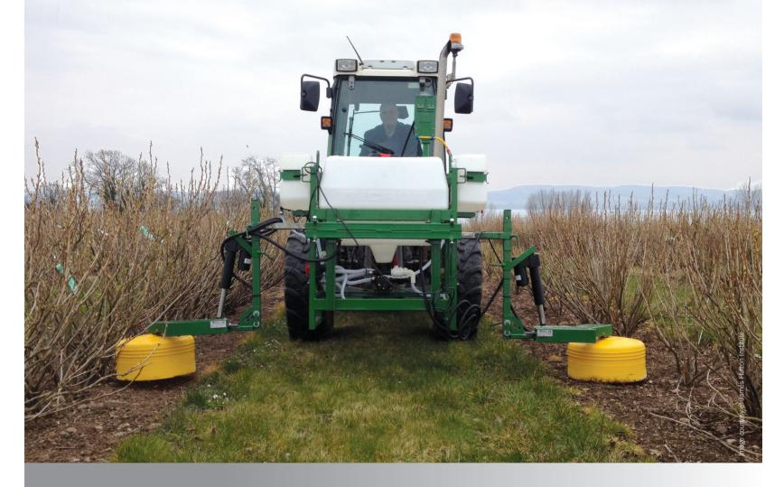
Spraydome shielded sprayers provide a safe, efficient and economical method of treating weeds round the base of mature bush crops and trees, as well as in amenity areas and other situations where a complete barrier to the spray is required.
