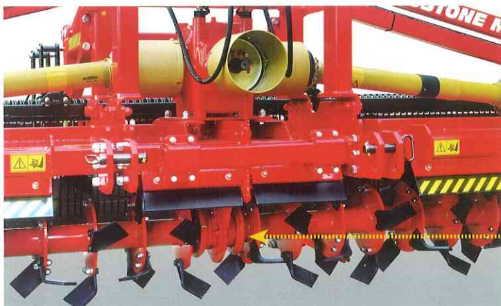
Supporto centrale. Central house bearing.
