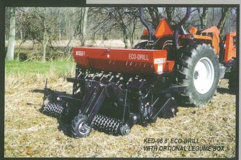
16" Straight Coulters slice the ground, followed by 13" Concave Openers to form a Seedbed Trench.
