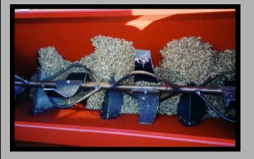
Our Optional, Patented "Positive Feed Agitator System" is designed to plant Native (Warm Season Grasses) This system is available in a second box, mounted alongside the standard Primary Seedbox. Units with box a Primary and a Warm Season Grass Box will plant virtually any seed variety wanted.
