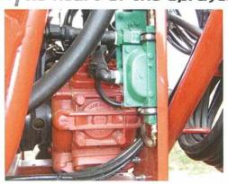
The HARDI® diaphragm pumps are designed for the application of crop protection products and liquid fertilize The ARROW is standard equipped with the HARDI® 363 HEAVY DUTY PUMP. The 363 HD is specially design for the abrasive chemicals used in orchard and vineyards HARDI® offers a 5 year prorated warranty on all pumps The HARDI® diaphragm pumps are:
