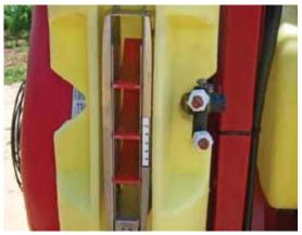
The IRIS application system allows for individual air adjustment as each outlet permits steep angling or even closing of the air supply, if necessary.
