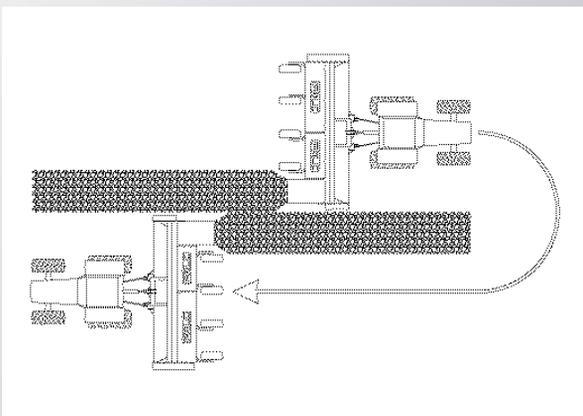
**FAST shredders** allow to shred and windrow stalks in one pass. Uniform windrows are ready for baling. It is possible to lay a second windrow adjacent to the first one (see the drawing). In a short time, it is easy to convert FAST into a standard shredder with unload of the chopped material on the ground.
