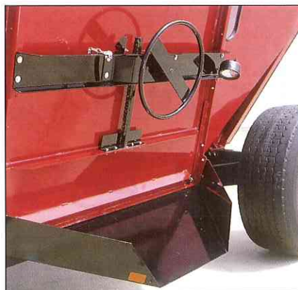
2.8:1 sprocket ratio door opener with roller guides and chute light
