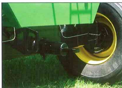
One piece reach pipe for pull through rear hitch design and safety chain support
